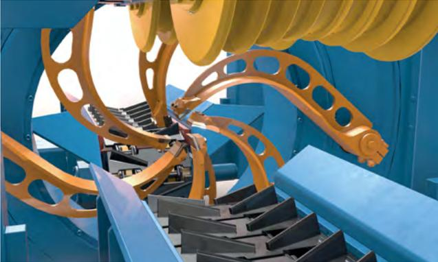
**Ring and rotary debarkers**, which utilize different technologies to remove bark from a log.
